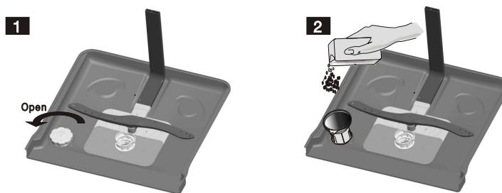
1. Remove the bottom basket and then unscrew the cap from the reservoir.
